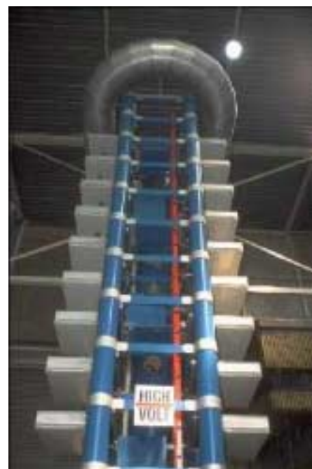
Impulse generator 2400 kV
