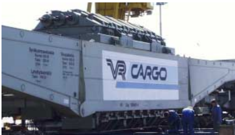
Transformer designed for special rail transport
