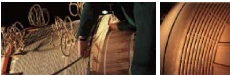
The use of epoxy bonded transposed cable and the application of axial cooling ducts increases the short circuit strength
