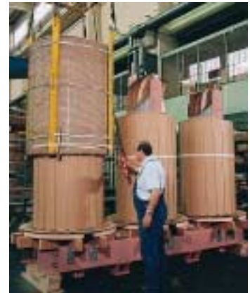
Assembly of Medium Power Transformer
