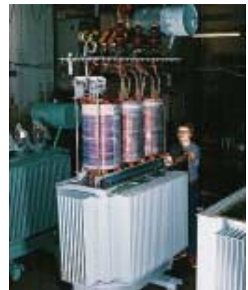
Assembly of Small Power Transformer
